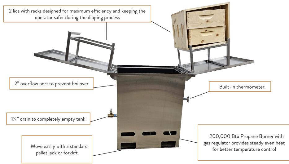
Production output 45 deep boxes/hour or 450 boxes/day...with 4-minute cycle Heavy-duty 14 ga and 11 ga 304 stainless steel construction
